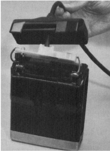
Fig. 2. Rear view of miners' cap lamp battery (lid removed).
